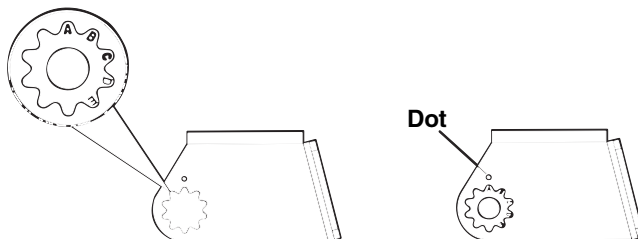
Align plastic ratchets in bracket.
