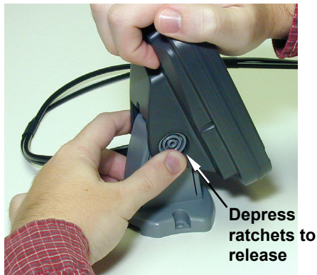
Cuda 300 quick release mounting bracket (left). Adjusting the viewing angle of a display unit (right).
