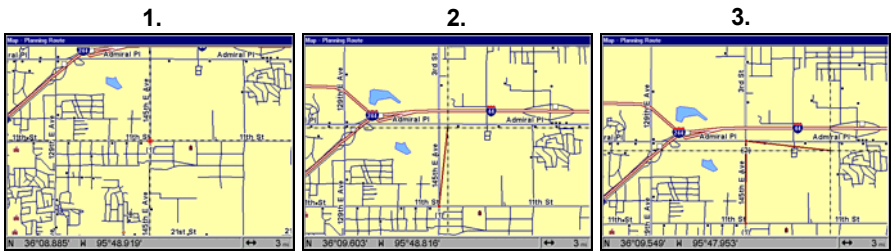
Route creation sequence, from left: (Fig. 1) Set route waypoint (1) at 11th St. & 145th Ave. (Fig. 2) Move cursor north to set point (2) at 145th & Admiral. (Fig. 3) With point (2) set, move cursor east to mark interstate on-ramp with waypoint (3). In figures 2 and 3, notice the rubber band line extending from the previously set waypoint to the cursor. This line will become the course for the route.
