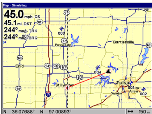
The overlay data on this map display includes, Ground Speed, Distance, Track and Bearing.
