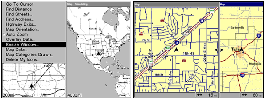
Map Menu with Resize Window command selected (left). Pressing → moves the centerline and enlarges the left window (right).
